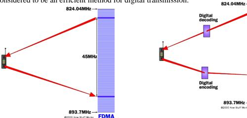
In FDMA, each phone uses a different frequency.
