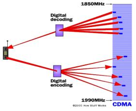
other on the channel, with each assigned a **unique sequence code**. CDMA is a form of **spread spectrum**, which simply means that data is sent in small pieces over a number of the discrete frequencies available for use at any time in the specified range.
